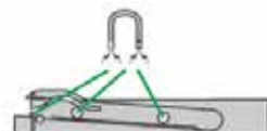
Magnets prevent the cutting insert from falling out of the tool holder during positioning
